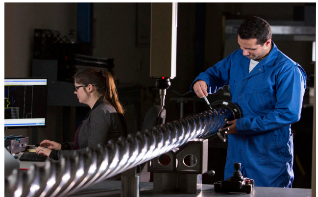
Precise measurement of a rotor profile
