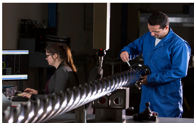
Precise measurement of a rotor profile
