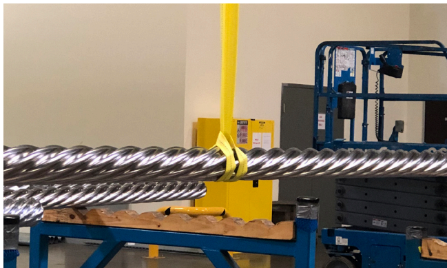
Use soft slings only when lifting rotors
