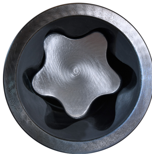
Cross section of power section
